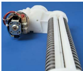
An enclosed transmission system protects the gear from dust and does not require lubrication or maintenance
